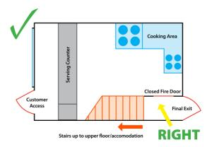
An enclosed staircase with fire resisting construction to ensure all exit routes are safe.
